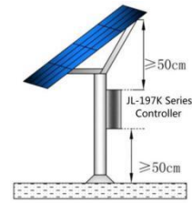
Figure 4. Control Box Location
